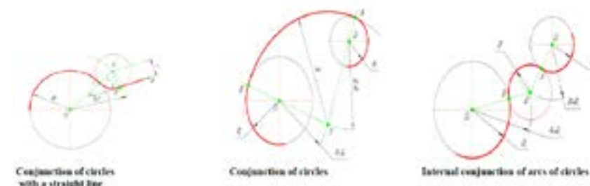
Figure 1 – Conjugation of circles (arcs) with a straight line conjugation of circles (arcs), internal conjugation of circular arcs
